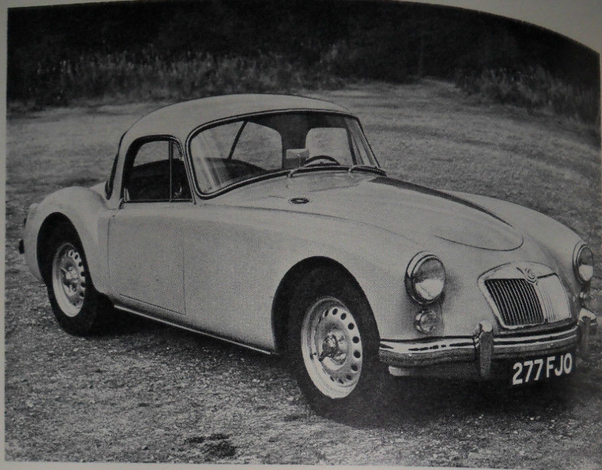
MGA Twin-cam, one of the most potent sports cars of today. The power unit develops 107 b.h.p. at 5,500 r.p.m.
