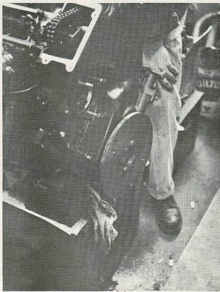
A degree wheel is a must if accurate valve timing is to be achieved on MG.
