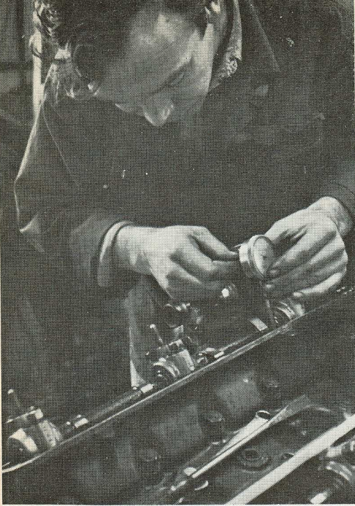
LEFT — Joe Virag checks out the valves with a dial indicator prior to disassembly of the engine. All timing was carefully checked during dismantling and assembly. ABOVE — Ports on exhaust side are huge and virtually straight through. No enlargement necessary but all ports were matched to manifolds and equalized in size.
