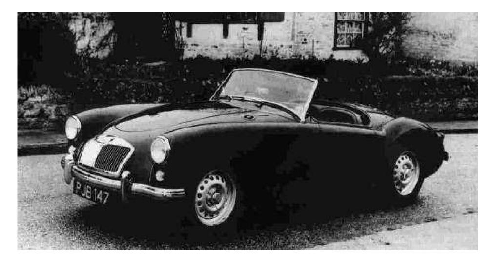
The 'Twin Cam' goes well with its o.h.c. engine and 120 m.p.h. speed, stops well with its disc brakes on all four wheels, and looks well with its aerodynamic body and knock-on disc wheels.
