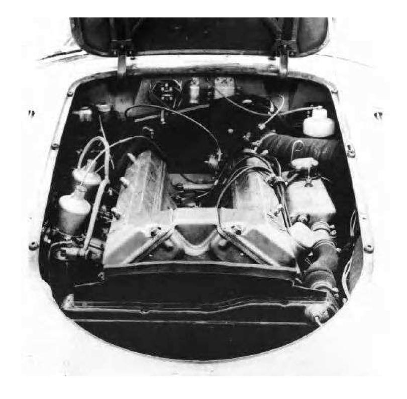
The polished aluminum camshaft covers distinguish the engine of the 'Twin Cam'. At left are the twin H6 S.U. carburetors and at right is the radiator header tank...
