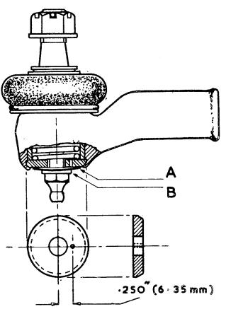
It is most important to ensure that only the correct fibre washer (Part No. ACH6173) is fitted. An ordinary commercial fibre washer must not be used.
