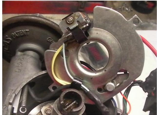
In distributors such as the DM2 where the two sensors are located on separate assemblies, a flexible thermal bridge consisting of soft copper wire braid may be attached to the two sensor supports to reduce their mutual thermal gradient. Even without this aid, the reference sensor correction reduces total vac error below 0.2CD between 0C and 80C and below 0.05CD over the cruising temp range.
