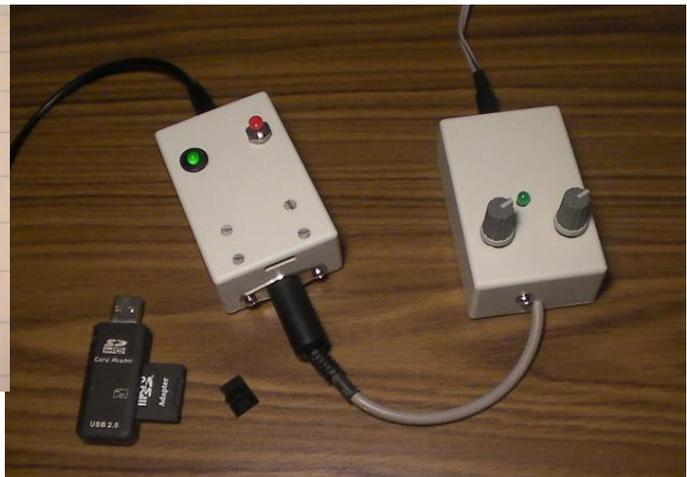
vehicle data logging and the USB adapter necessary if a micro-SD slot is not present in the host data analysis computer.
