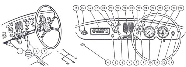
1, Headlamp dipswitch. 2, Gear lever. 3, Handbrake. 4, Bonnet catch release. 5, Windscreen washer button. 6, Heater air-intake control. 7, Heater temperature control. 8, Demister control. 9, Water thermometer. 10, Dynamo charge warning light. 11, Headlamp main beam indicator
