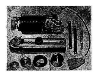
Supercharger with idler assembly, intake manifold, exhaust manifold and carburetor assembled (fuel bolt, fibre washers and spring attached to carburetor.)
